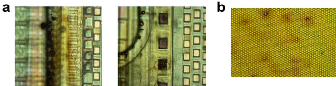
Figure 4–12: CMOS-HDMEA damage. a. Images showing water marks on the bond pads of the CMOS-HDMEA. This occurrence happens when the epoxy coverage lifts and creates a tiny gap for water to seep to the bond pads and bond wires, which should otherwise be protected from liquid. b. Further indication of damage on the microelectrodes.
